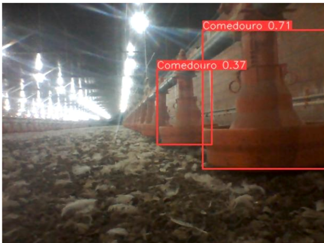
Fig. 3. Detection of feeders by computer vision. Source: Cardoso et al. (2023).
